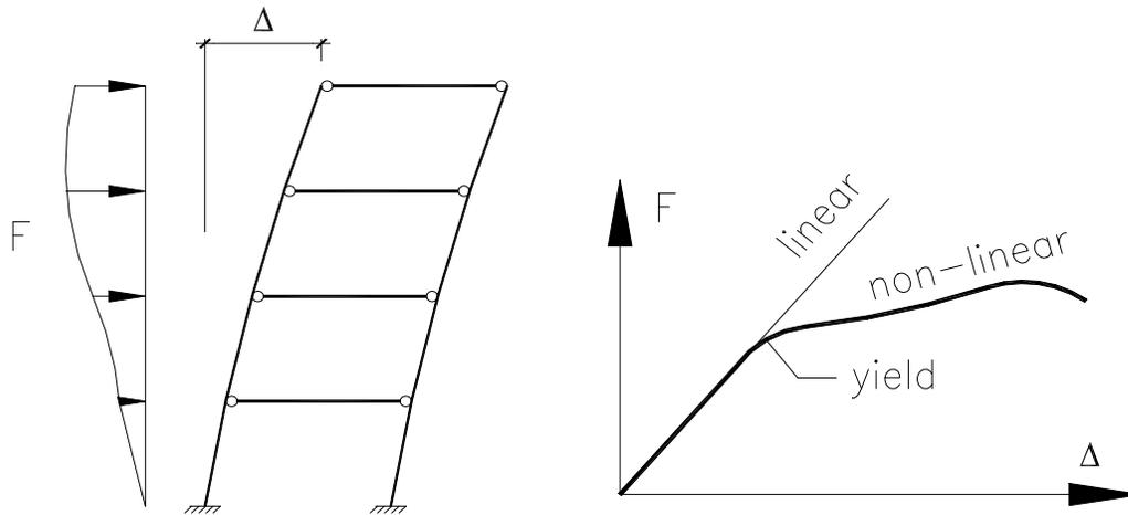
Ductility is the measure of how much plastic strain a single element or whole structure can experience before it is damaged to a point where it can no longer sustain loading. It is usually expressed as a multiple of the yield strain. There are various options to suitably account for ductility (i.e. a nonlinear response) in analysis.
